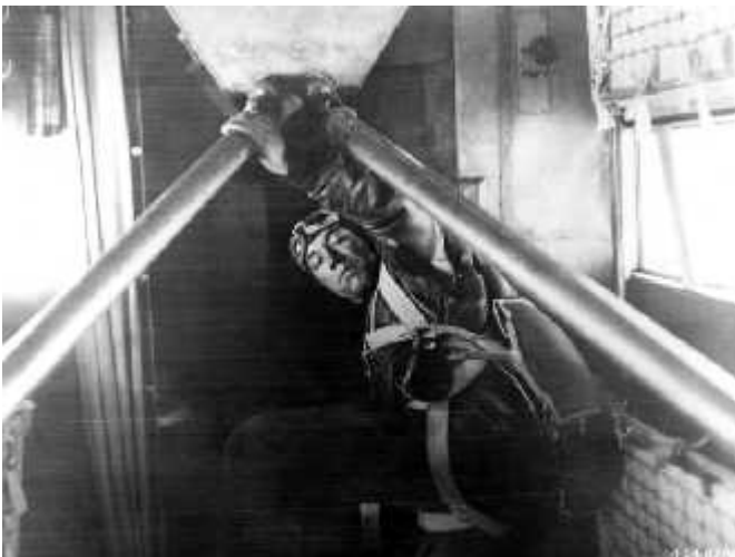
Lt. Elwood Quesada adjusts an aircraft gas line during a 1929 operation dubbed Question Mark.
